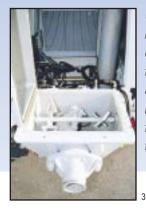
Unique to the TK 25 is that the S-valve can be adjusted from the outlet end. In addition, its hopper lid conveniently opens for easy accessibility to components.
